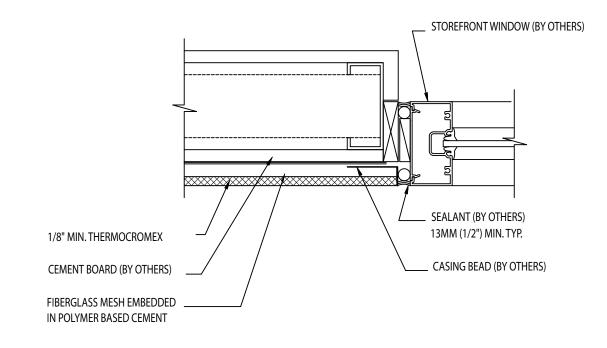
NOTE: All joints of cement board must be treated with 4" fiberglass mesh embedded in polymer based cement.
